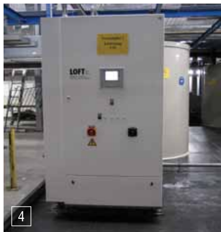
5 - Evaporator for the zinc-phosphating baths
