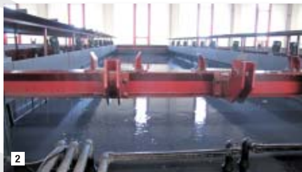
1 View of the new Brantner coating plant implementing the Aquence™ autodeposition chemical process – an aqueous organic solution forming a uniform coating film even on the most complex shapes.
